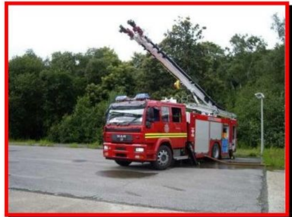
Integral water tank and fire pump offer a Quint style multi-functional vehicle
