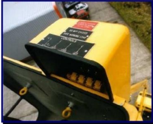
Cage hydraulic controls, showing the 2 x Safety Harness anchor points for the Operators
