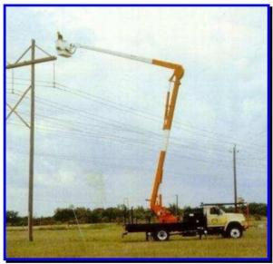
THE RANGER INSULATOR WASHER BOOM TRUCK mounts onto a wide range of chassis types to suit all applications. It is available with a skid mounted insulator washer pump and engine module and removable water storage tank up to 10,000 litre capacity with 4 main boom options at 14; 16; 20.5 and 22m working heights.
