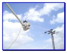
Two-man fully insulated basket and boom for washing safely at heights up 22m and on live lines up to to 500kV with the Translink proven insulator washer system.
